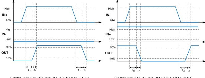
(PWM input to IN+ pin, IN- pin tied to GND)
